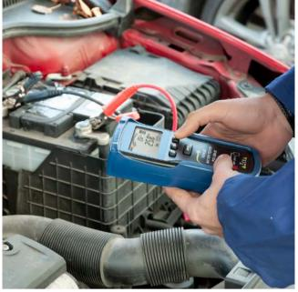
Car measuring device for 12 V and 24 V starter batteries / starter and charging circuit measurement / LC display / rubber holster / easy handling
